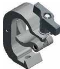
CLP-P589 weight = 0.50 kg Clamp (48-51 mm) | SWL 350 kg (SF 8:1)
