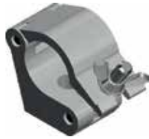
CLP-P587 weight = 0.57 kg Clamp side entry (48-51 mm) | SWL 780 kg (SF 8:1)
