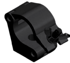
CLP-P587B (Black) weight = 0.57 kg Clamp side entry (48-51 mm) | SWL 780 kg (SF 8:1)
