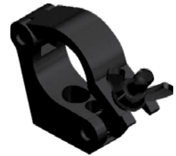
CLP-P588B (Black) weight = 0.37 kg Clamp slim side entry (48-51 mm) | SWL 410 kg (SF 8:1)
