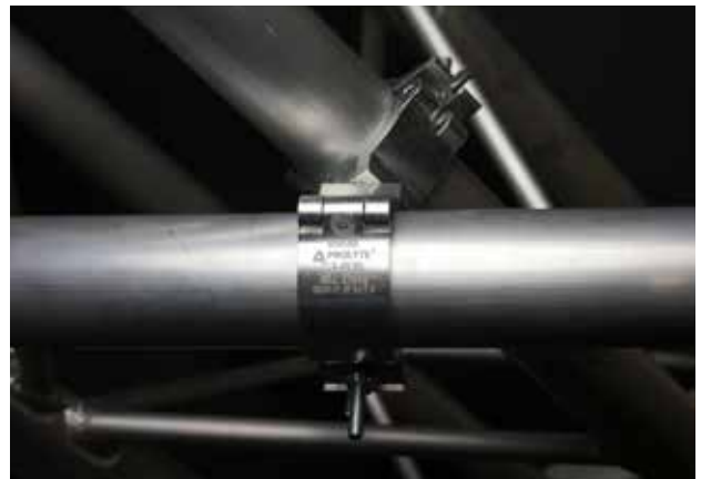
CLP-P536L weight = 0.27 kg Swivel coupler (48-51 mm) SWL 230 kg (SF 8:1)
