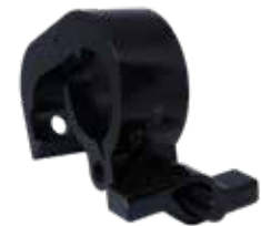
CLP-P589B (Black) weight = 0.50 kg Clamp (48-51 mm) | SWL 350 kg (SF 8:1)
