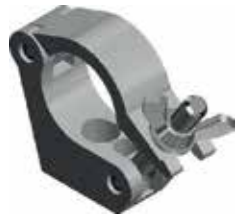
CLP-P588 weight = 0.37 kg Clamp slim side entry (48-51 mm) | SWL 410 kg (SF 8:1)
